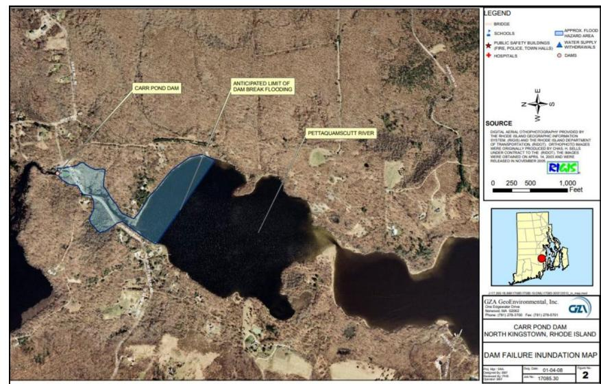
**Attachment 1 - Figure 11: Dam failure inundation map for Carr Pond Dam (No. 513)**
